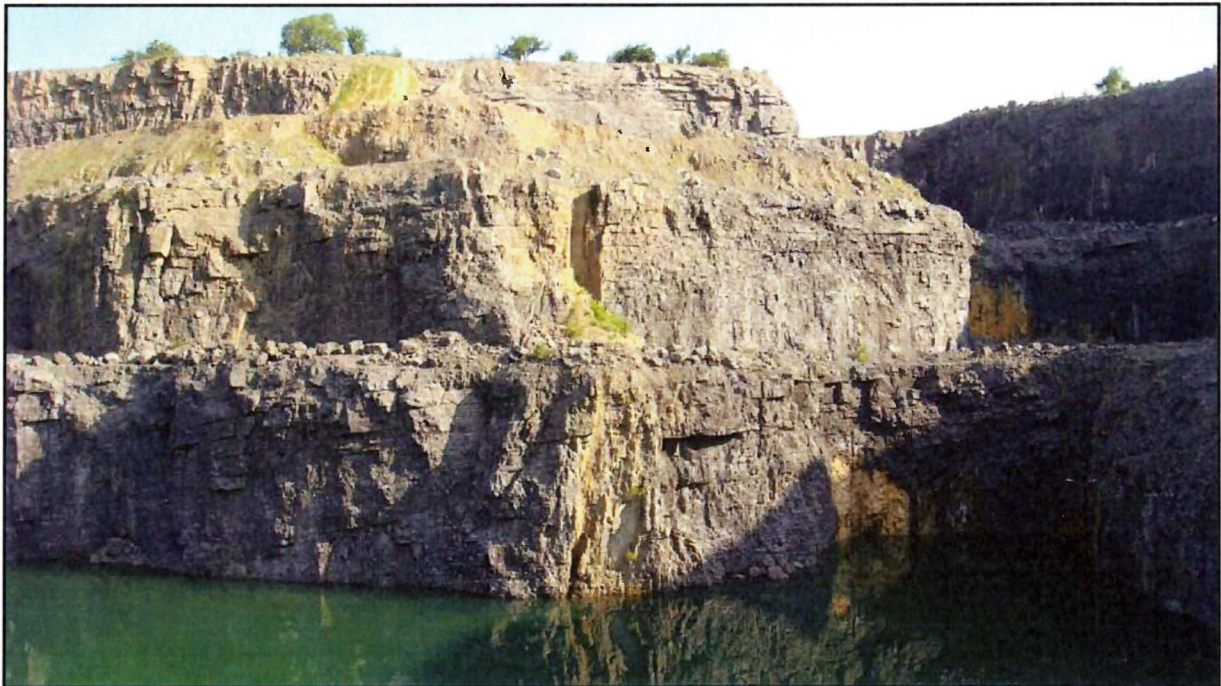
Plate 7-14: Large sub-vertical fault in east of quarry
